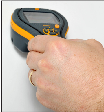
Figure 2: Using the Pin Moisture Meter
