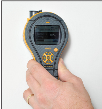
Figure 3: Taking Relative Moisture Readings
