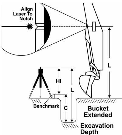
Place the laser in a location where receiver can pick up the beam, and turn it on.
